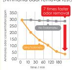
We used nonwoven filter fabric kneaded with fine Todomatsu powder. It was confirmed that ammonia that causes bad smell was removed 7
