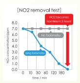
We used nonwoven filter fabric kneaded with NO2 that causes environmental pollution was rendered harmless in 3 hours.
