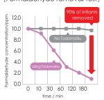
We used nonwoven filter fabric kneaded with fine Todomatsu powder. It was confirmed that formaldehyde that is an irritant found in adhesive and paint used around the house was reduced by 90% in 3 hours.
